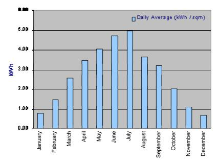
Figure 13 Daily average power output of a solar hot water system in Scotland. Source: Energy Systems Research Unit, University of Strathclyde<sup>200</sup>
