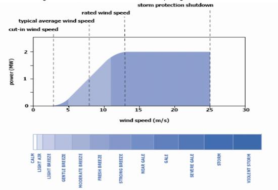
Figure 12 Typical power curve of a wind turbine. Source: BWEA<sup>144</sup>
